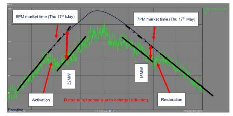
Demand reduction due to voltage reduction Test conducted on 17<sup>th</sup> May 2018 for a 2 hour period.
